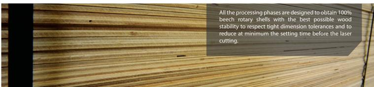
The temperature and humidity parameters during the curving process are strictly controlled for each range of shell diameter.
